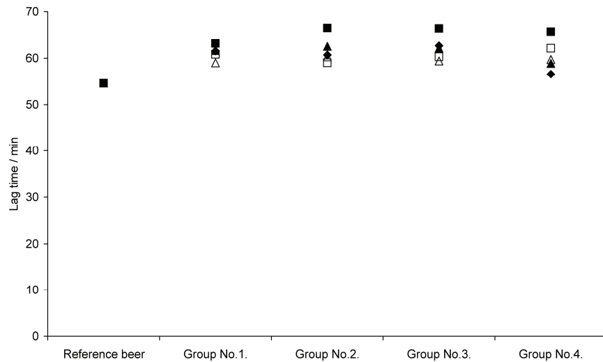
Fig. 1. Lag time values when vitamin E and C were added to packaged beer with the original and lower pH: ◆ only vitamin E added – normal pH; ■ only vitamin C added – normal pH; ▲ only vitamin C added – lower pH value; △ vitamin E and C added – normal pH; □ vitamin E and C added – lower pH value.
